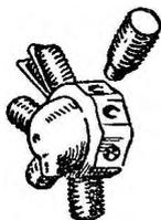
Fig. 6.—The crankcase of the metal engine is filed from a brass rod and the cylinders are small brass bolts.
